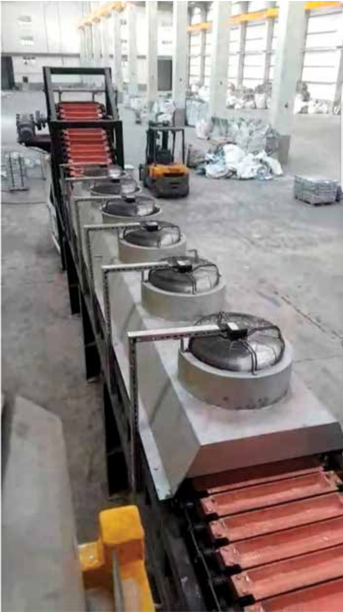
Ingot casting mashines. Equipment example from ALM Company
