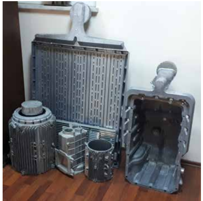
Some examples of aluminum alloy castings obtained on the proposed HPDC machines
