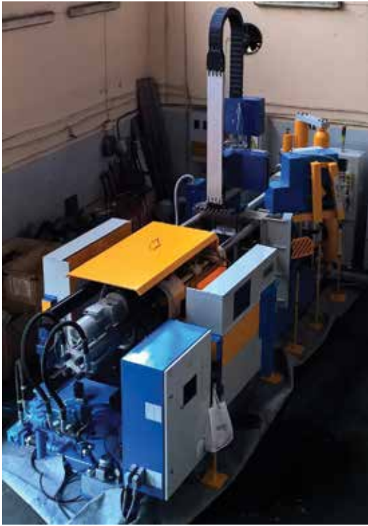
High pressure die casting machine with a cold chamber with a locking force of 200 tons with automatic melt pouring and die lubrication systems
