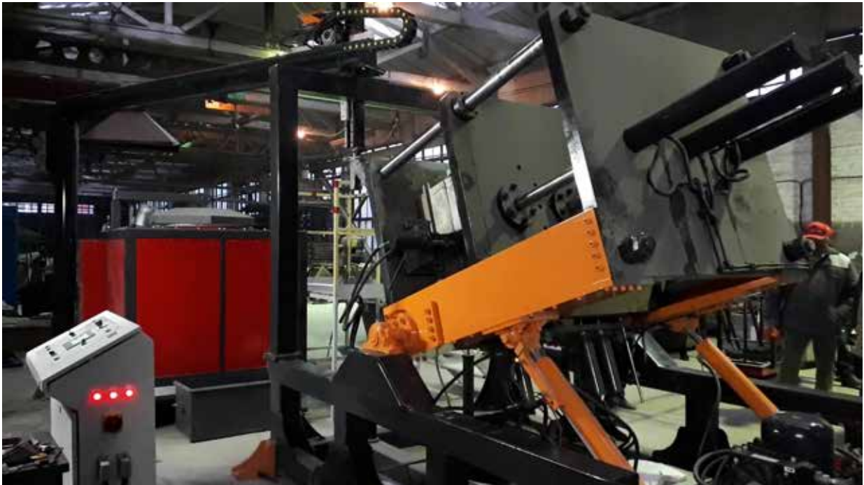
Automatic gravity die casting cell based on tiltable gravity casting machine SA-Foundry ALG-1500*1300
