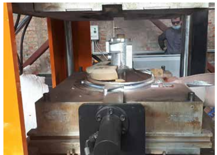
The resulting casting of the aluminium pump body before being ejected from the die
