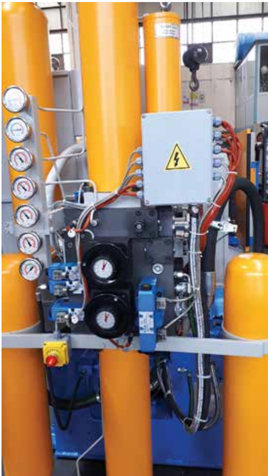
Unit for adjusting the pressing system of the HPDC machine with a locking force of 300 tons
