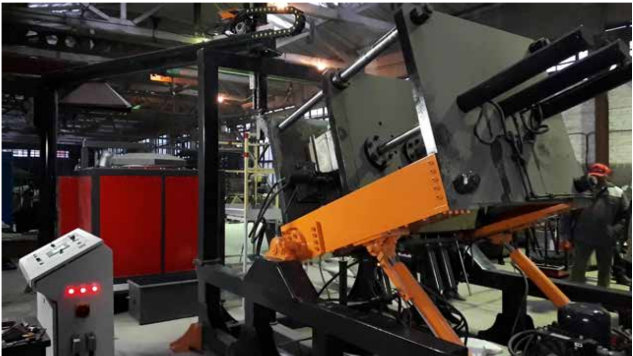
Automatic gravity die casting cell based on tiltable gravity casting machine SA-Foundry ALG-1500*1300
