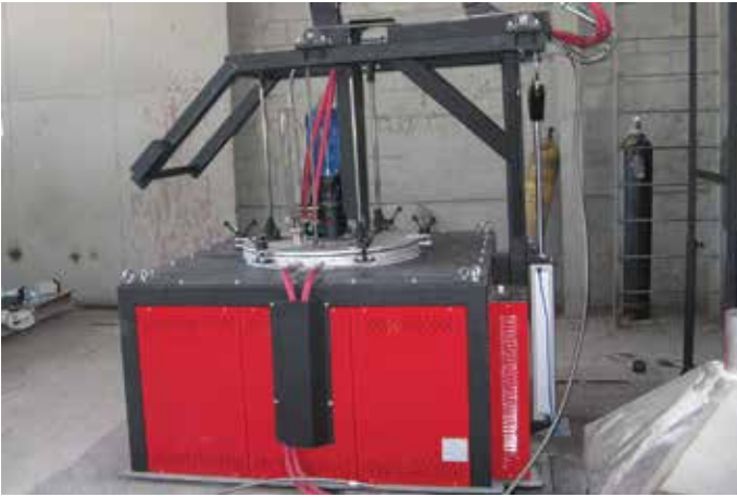
Shaft furnace with gastight retort and atmosphere circulation for heat treatment in protection atmosphere and thermochemical treatment of metals
