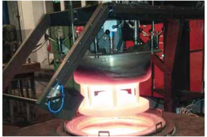
Shaft furnace with gastight retort and atmosphere circulation for heat treatment in protection atmosphere and thermochemical treatment of metals
